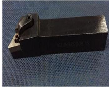
**Gambar 1.** *Tool Holder* DNMG MDJNR2020K
