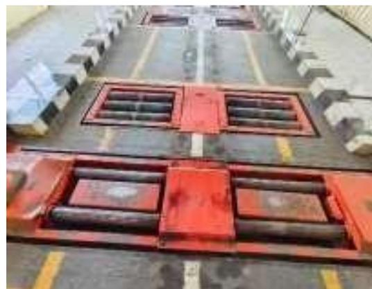
**Gambar 2.** Alat Uji Brake Tester
