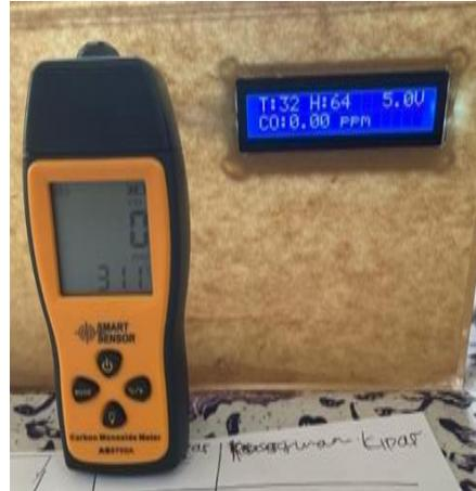
**Gambar 3.** Smart Sensor Carbon Monoxide Meter AS8700
