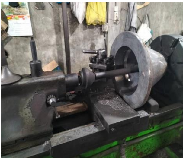
a. Proses finishing
